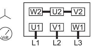
Double star connection, multi-voltage motor with 9 terminals (low voltage):
