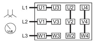
Delta connection, multi-voltage motor with 12 terminals (middle voltage):
