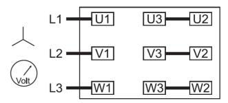
Double star connection, multi-voltage motor with 12 terminals (low voltage):
